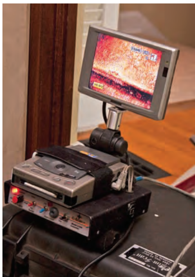
Photos by Brandon Smith | Joe Sauter of Your Chimney Sweep uses a special camera to inspect the flue liner of a chimney in an Indianapolis home.
